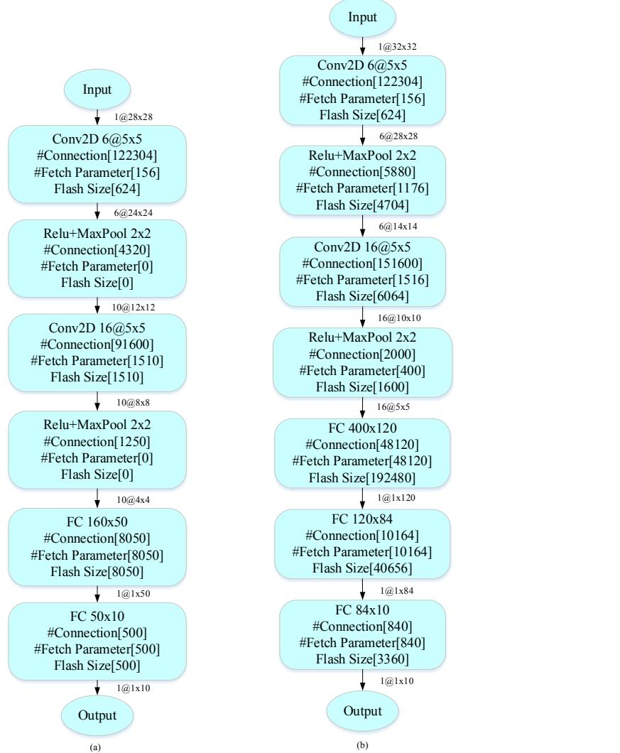
**Figure 3:** Model architectures found with the best test accuracy on MNIST-10(a), and compared the original LeNet-5 structure(b), each node in the graph are annotated with connection, parameter and flash size, # represents the number of corresponding objects, and the values in square brackets show the quantities
