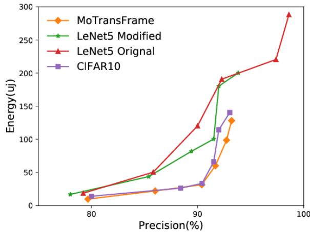
**Figure 6:** Comparison of energy consumption with different CNN architectures
