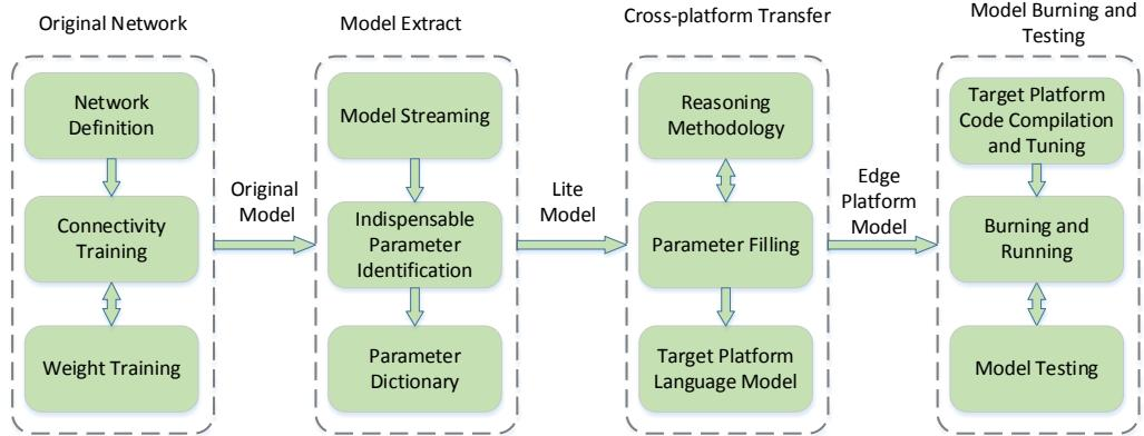
**Figure 2:** Four-stage pipeline for Model Transfer Framework
