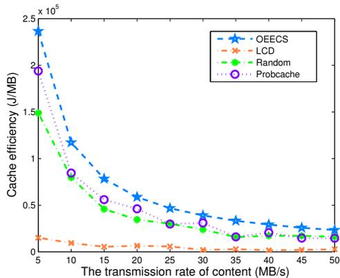
Fig. 9: The effect of  $R$  on cache efficiency:  $m=1000$ ,  $c=50$ ,  $P_c=10$ .
