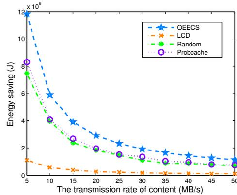
Fig. 7: The effect of  $R$  on energy saving:  $m=1000$ ,  $c=50$ ,  $P_c=10$ .
