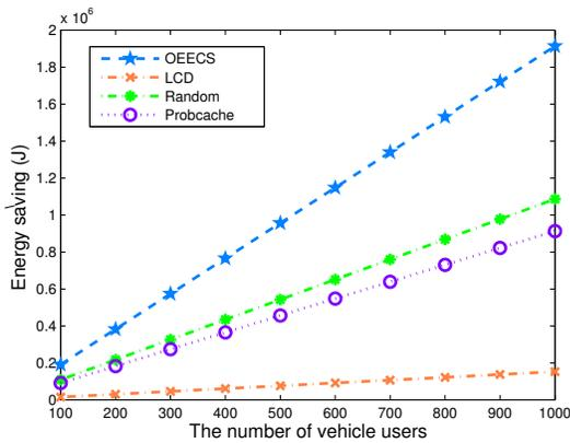
Fig. 5: The effect of the number of vehicle users  $m$  on energy saving:  $c=50$ ,  $P_c=10$ .
