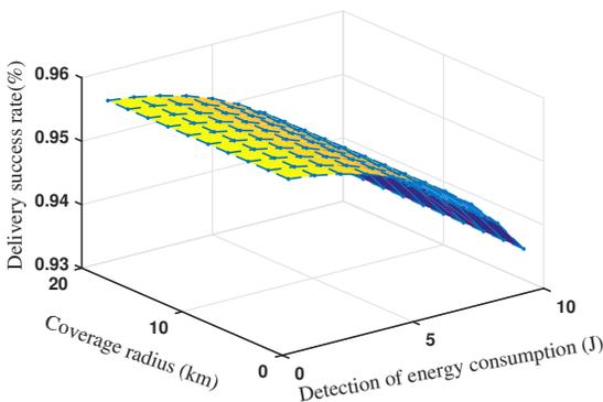
Fig. 12: The effect of  $P_c$  and coverage radius  $r$  on delivery success rate.
