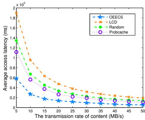
Fig. 11: The effect of  $R$  on average access latency:  $m=1000$ ,  $c=50$ ,  $P_c=10$ .
