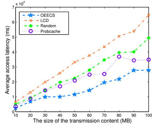
Fig. 10: The effect of  $c$  on average access latency:  $m=1000$ ,  $P_c=10$ .
